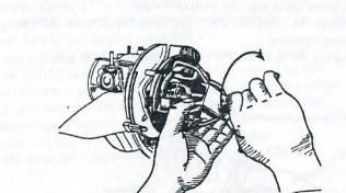
When reassembling, lock the crankshaft with the locking pin. Position the stator complete with its bearing on the crankshaft and insert the three securing screws (the two inside the stator complete with blank fan-lock washers).
